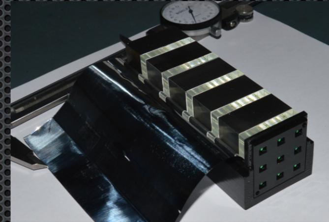
One SiPM for each fiber in the back of each module. Summed signals (9 SiPM per ADC) to reduce cost
