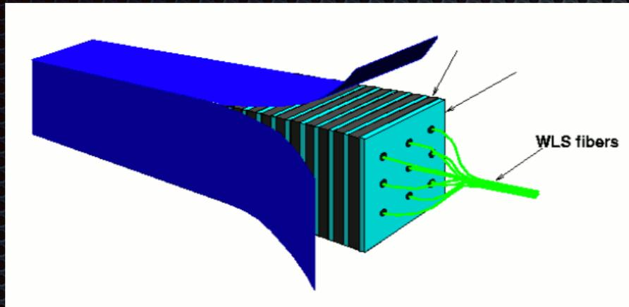
Cheap, fast ( $<10$  ns) and radiation hard (ENUBET needs 1.3 kGy: not critical) is the base unit of ENUBET
