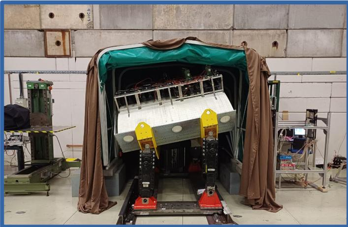
Assembled in INFN-Legnaro, charged beam tested at CERN several times under NP06/ENUBET experiment
