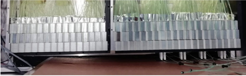
Fig. 7. Lateral readout prototype tested in 2018, with integrated photon veto (bottom right).
