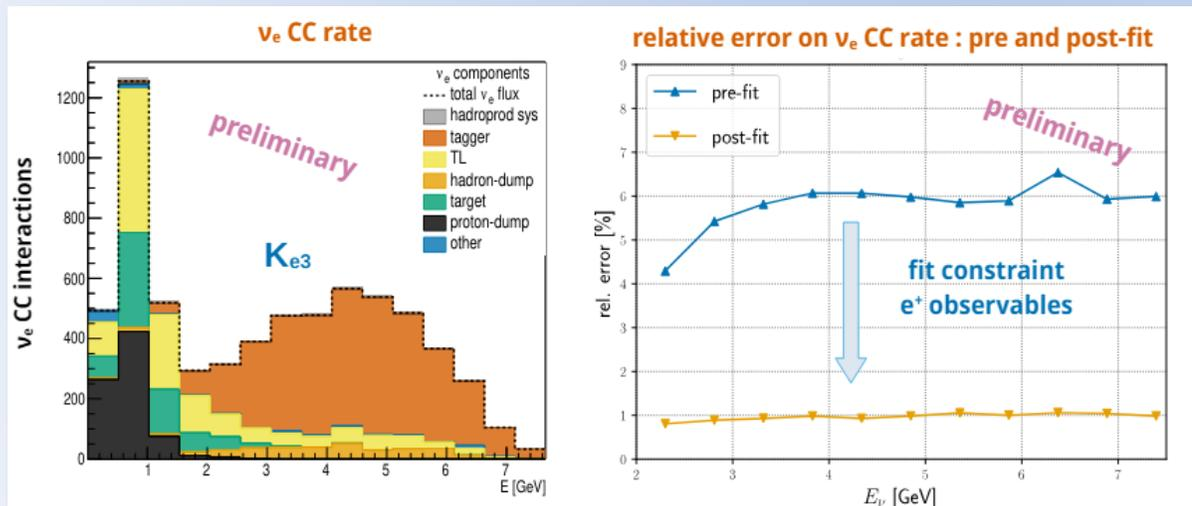
The flux uncertainty for  $\nu_\mu$  and  $\nu_e$  **drops from 6% to 1%** using positrons only
