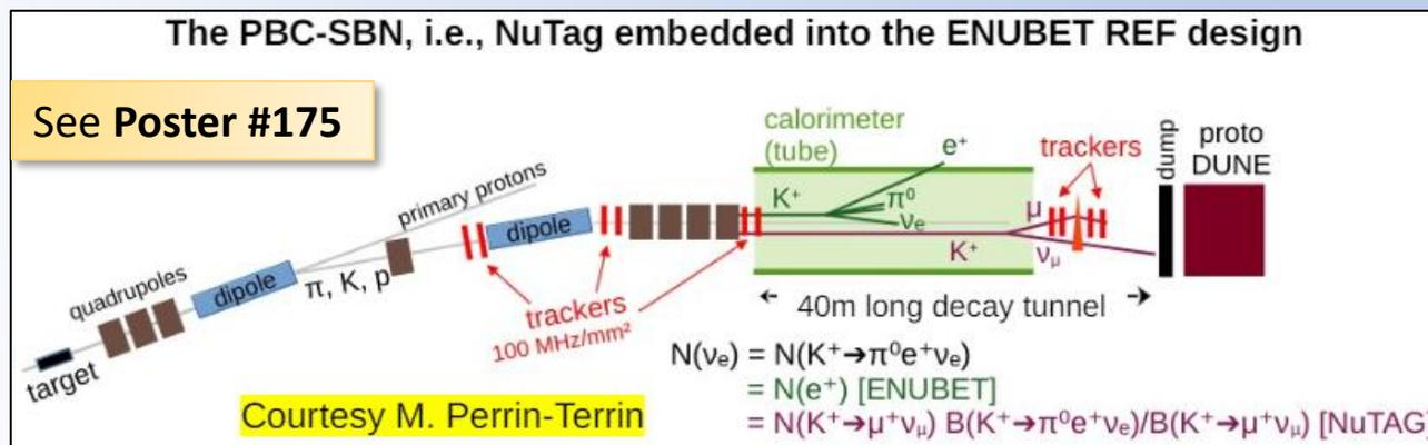
We can do much better exploiting the NuTAG concept, i.e. adding silicon trackers in the beamline to tag the neutrino parent. **Expected neutrino energy resolution: 1%**
