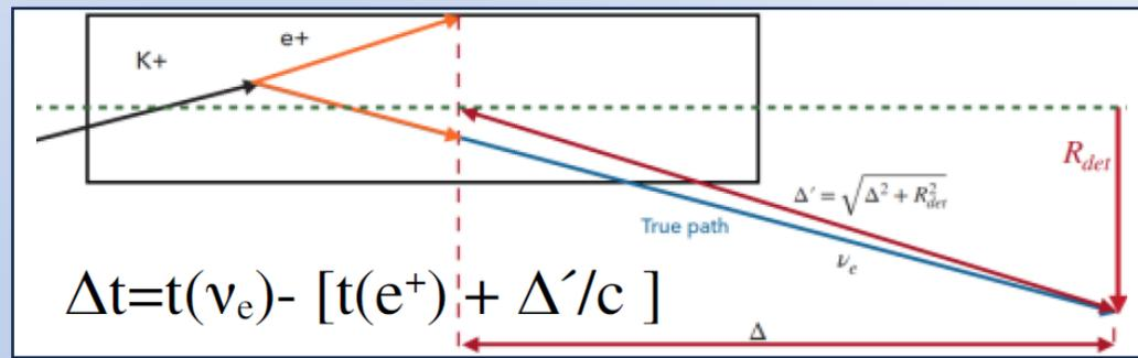
Assuming a time resolution  $\delta t = 200$  ps for both the  $\nu$  detector and the tunnel instrumentation (ENUBET t0-layer with PICOSEC Micromegas)
