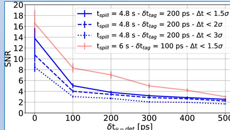
**Signal to noise ratio of tagged  $\nu_e$ - $e^+$  pairs as a function of the neutrino detector time resolution**
