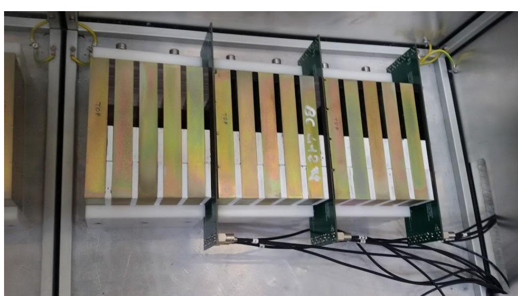
Shashlik calorimeter prototype
