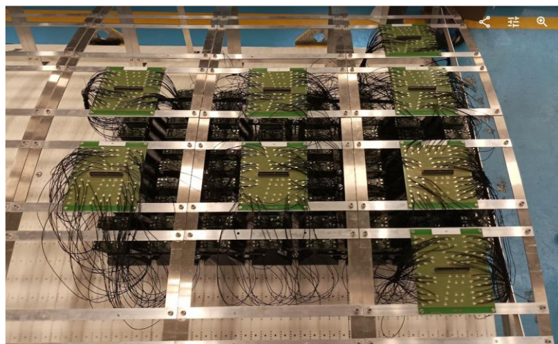
Custom interface board to connect 5 FEB (60 ch) to 1 A5202 (64 ch)
