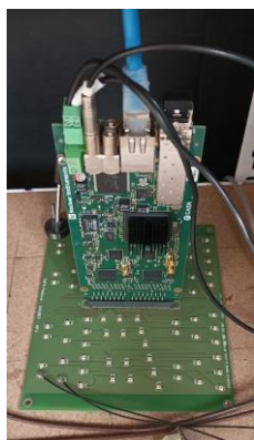
Front-End Board (SiPMs + Low V)
