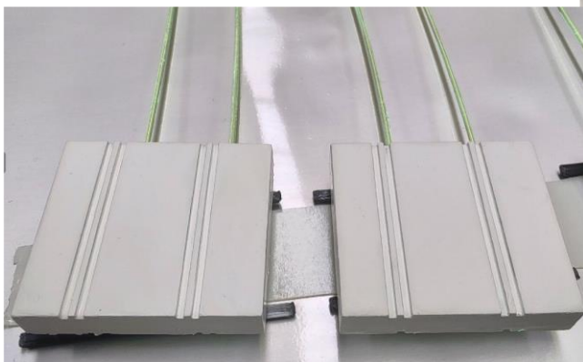
Tile painting (EJ-510 TiO 2 reflecting painting)
