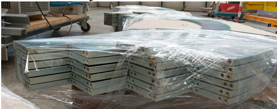
Machined iron for calorimeter absorber layers
