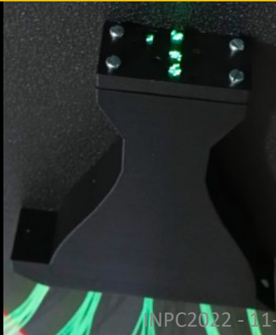
Fiber concentrator (bundling/routing to SiPMs)
