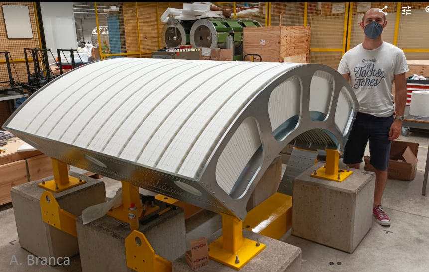
Fiber concentrator (bundling/routing to SiPMs)
