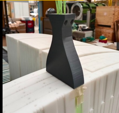
Fiber concentrator (bundling/routing to SiPMs)
