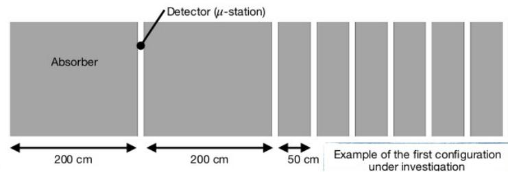
The most upstream (hottest) detector needs to cope with a muon rate of  $\sim 2$  MHz/cm<sup>2</sup> and about  $10^{12}$  1 MeV-n<sub>eq</sub>/cm<sup>2</sup>.
