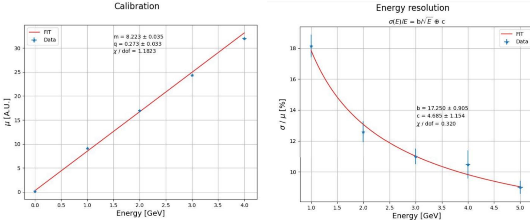
Figure 10: Linearity and energy resolution for electrons.
