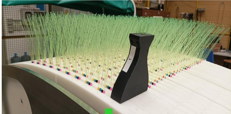
bundling of the WLS fibers with 3D printed “fiber concentrators”+ in situ polishing
