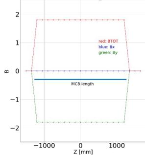
Standard B vs Z profile: MCB\_std at  $x = 0, y = 40$
