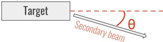
Maximum angle within magnets acceptance and heat endurance:  $1^\circ$
