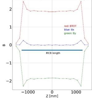
Standard B vs Z profile: MCB\_std at  $x = 0, y = 0$
