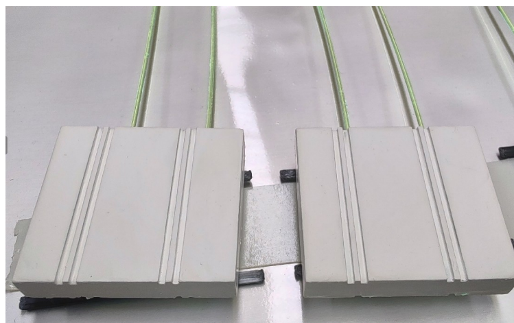
Tile painting (EJ-510 TiO 2 reflecting painting)
