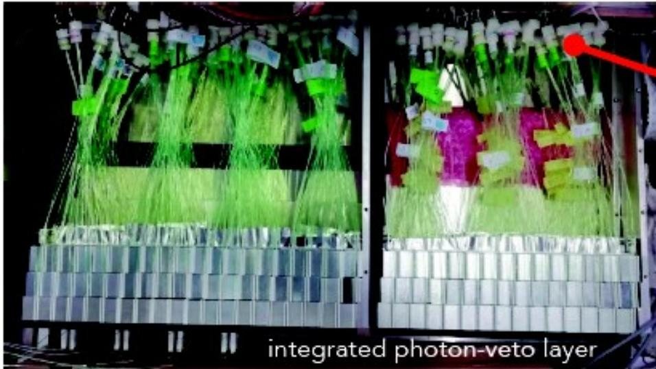
Large area (4x4 mm<sup>2</sup>) SiPM for 10 WLS (one LCM)
