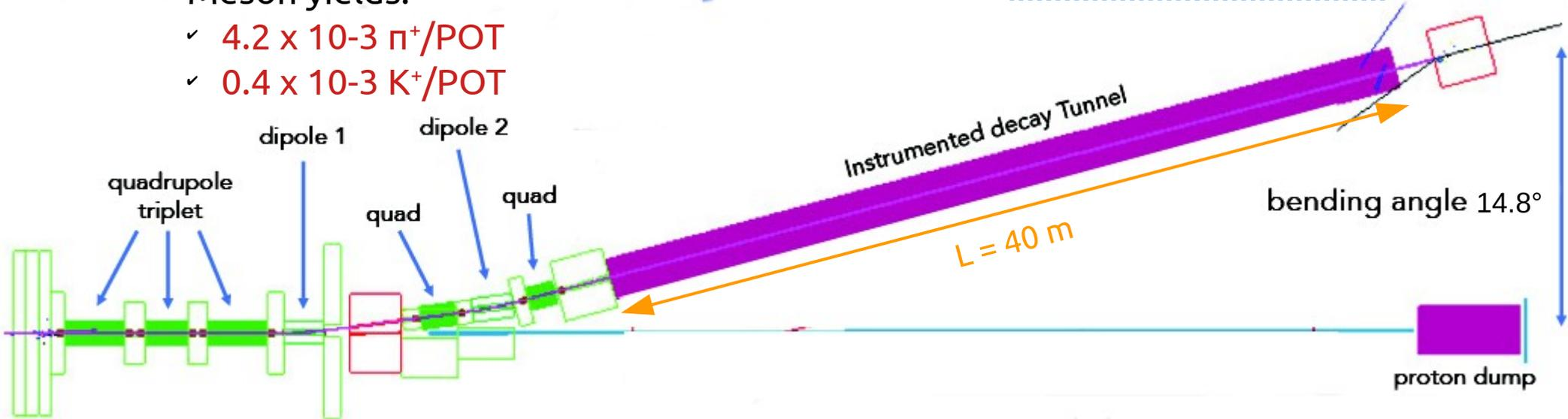
Collimators and shieldings tuned to keep under control backgrounds in the tunnel while retaining large enough meson yields
