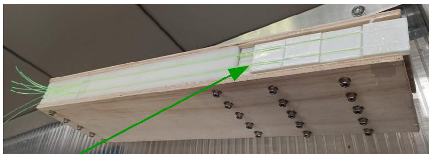
**WLS** collecting light from each module through grooves on the frontal face of scintillator tiles
