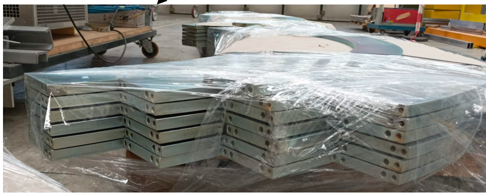
Machined iron for calorimeter absorber layers
