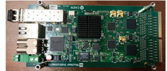
Commercial read-out boards (CAEN A5202)
