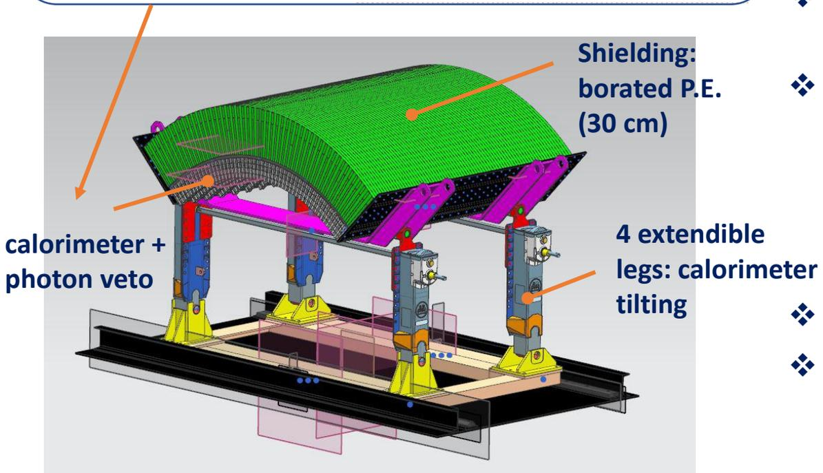
❖ Detector prototype under construction, to demonstrate:
