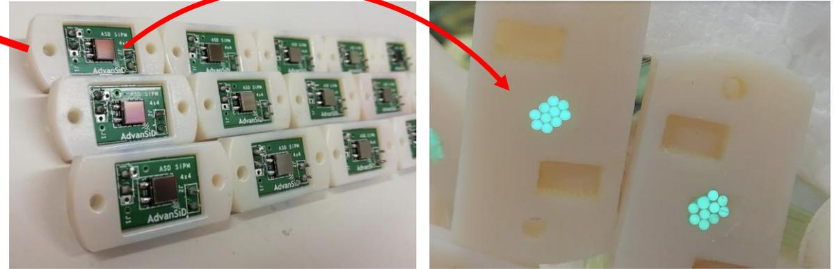
SiPMs installed outside of calorimeter, above shielding: avoid hadronic shower and reduce (factor 18) aging
