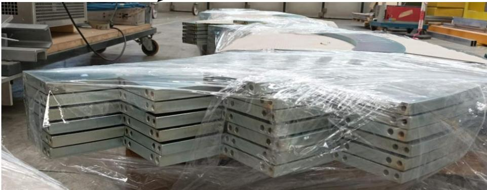
Machined iron for calorimeter absorber layers
