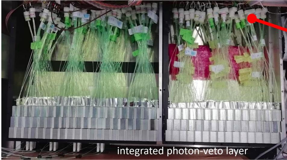
Large SiPM area (4x4 mm<sup>2</sup>) for 10 WLS readout (1 LCM)
