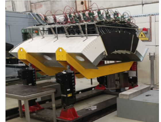
The NP06/ENUBET prototype of a section of the decay tunnel (1.65m length, 90° azimuthal coverage) tested at CERN PS T9.
