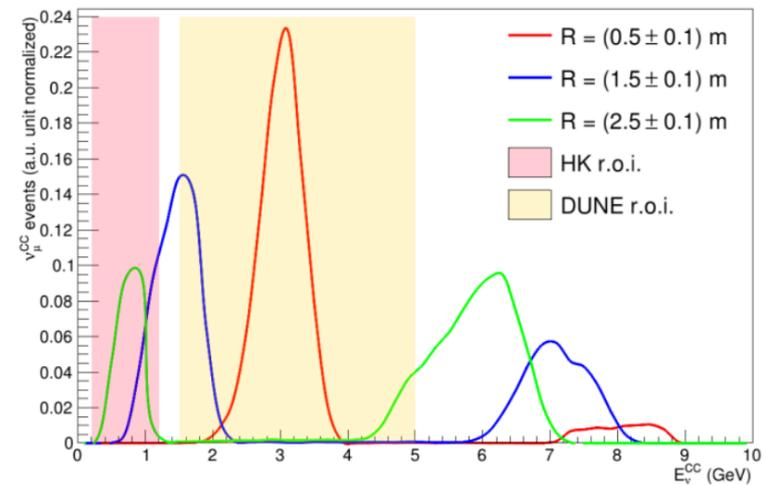
Initial neutrino energy inferred from the measurement of the neutrino interaction vertex distance with respect to the axis of the decay tunnel
