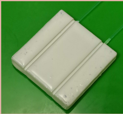
New solution (demonstrator): fibers collect the scintillation light frontally (fibers 1.5 cm apart)
