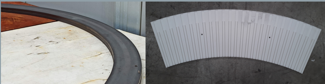
Iron layers and borated polyethylene layers available at INFN-LNL for assembly
