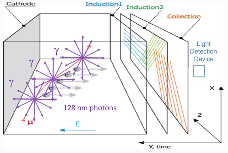
The DUNE LArTPC will be the largest liquid argon detector ever built. Noble liquid particle detectors normally use both the prompt scintillation light and the charge ionisation signals to perform event reconstruction.
