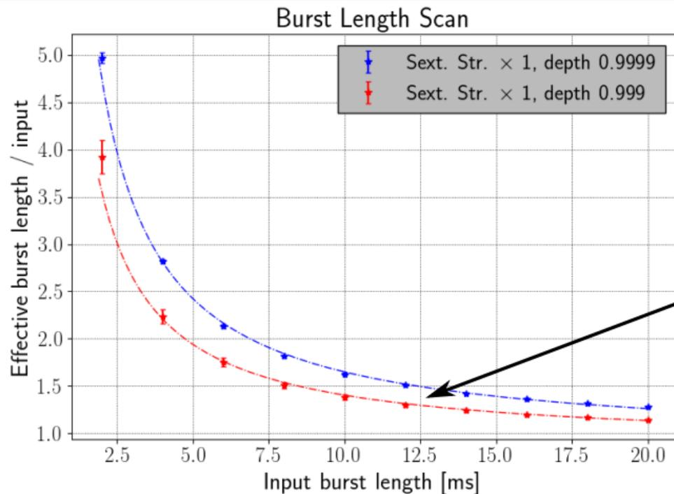
For a fixed simulated demanded burst length, tune speed in non-extraction regions defines a range of achievable effective burst lengths (i.e. between red and blue)
