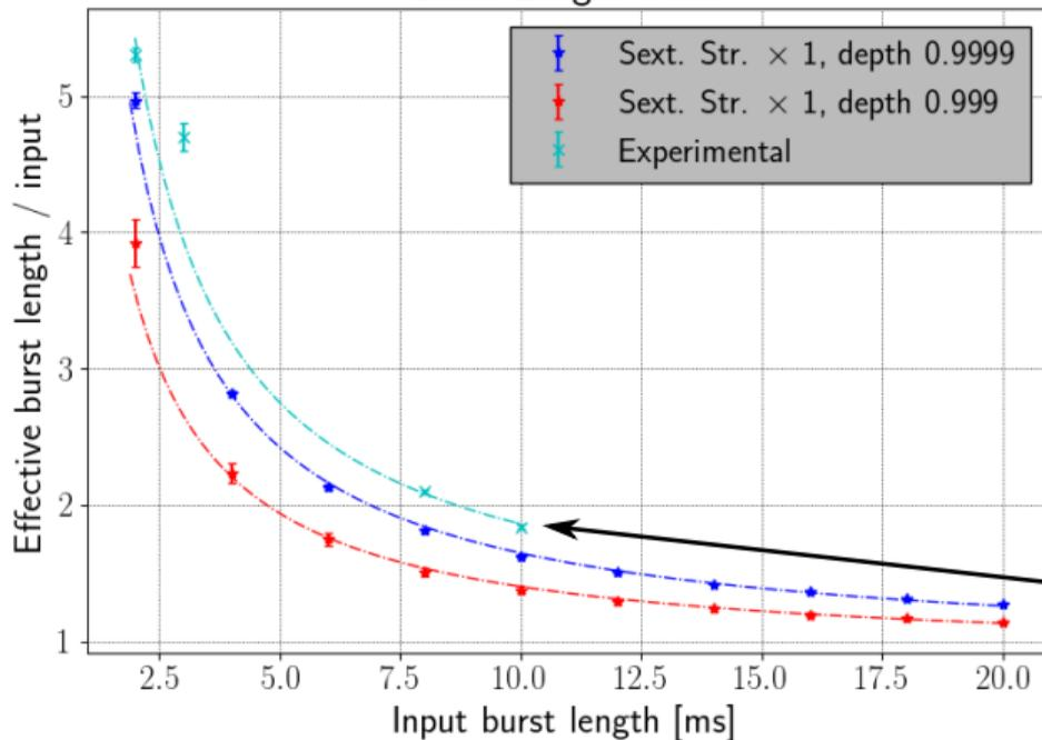
For a fixed simulated demanded burst length, tune speed in non-extraction regions defines a range of achievable effective burst lengths (i.e. between red and blue)
