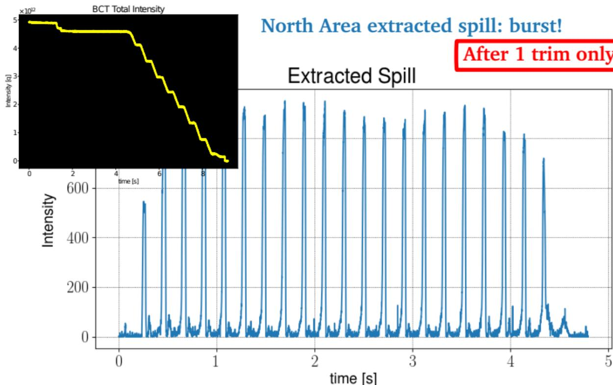
Measured spill in extraction TL with secondary emission foil.
