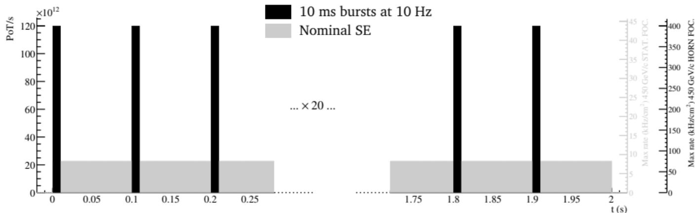
From simulations [1]:  $\sim \times 10$  neutrino flux increase in burst mode
