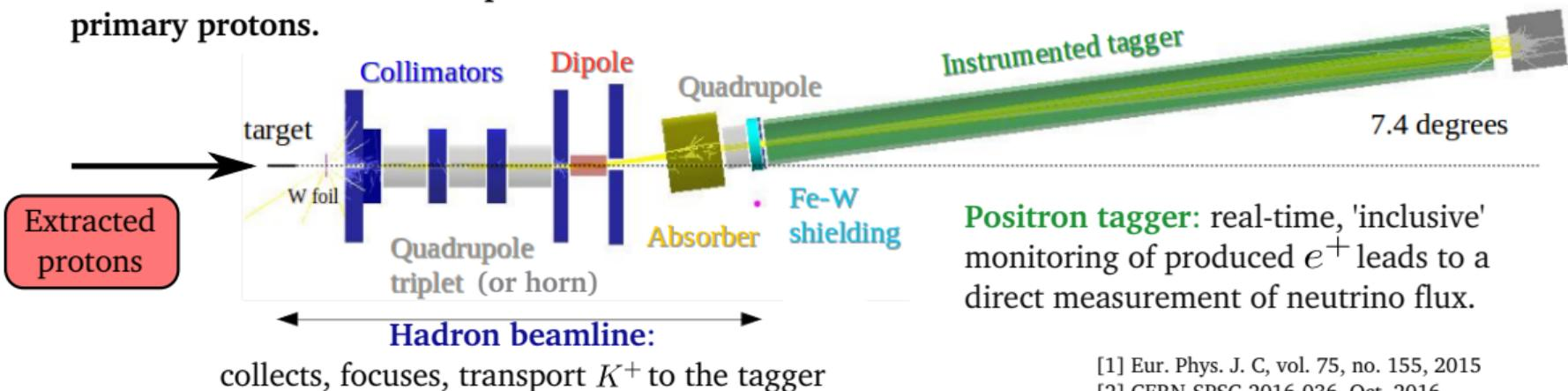
**Positron tagger:** real-time, 'inclusive' monitoring of produced  $e^+$  leads to a direct measurement of neutrino flux.
