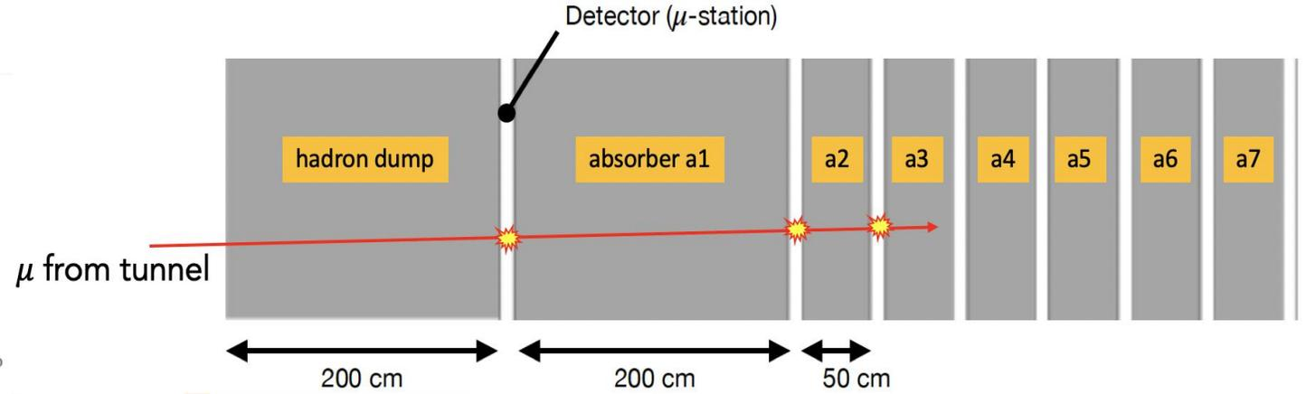
**Hottest detector (upstream station):** cope with  $\sim 2$  MHz/cm<sup>2</sup> muon rate and  $\sim 10^{12}$  1 MeV-n<sub>eq</sub>/cm<sup>2</sup>
