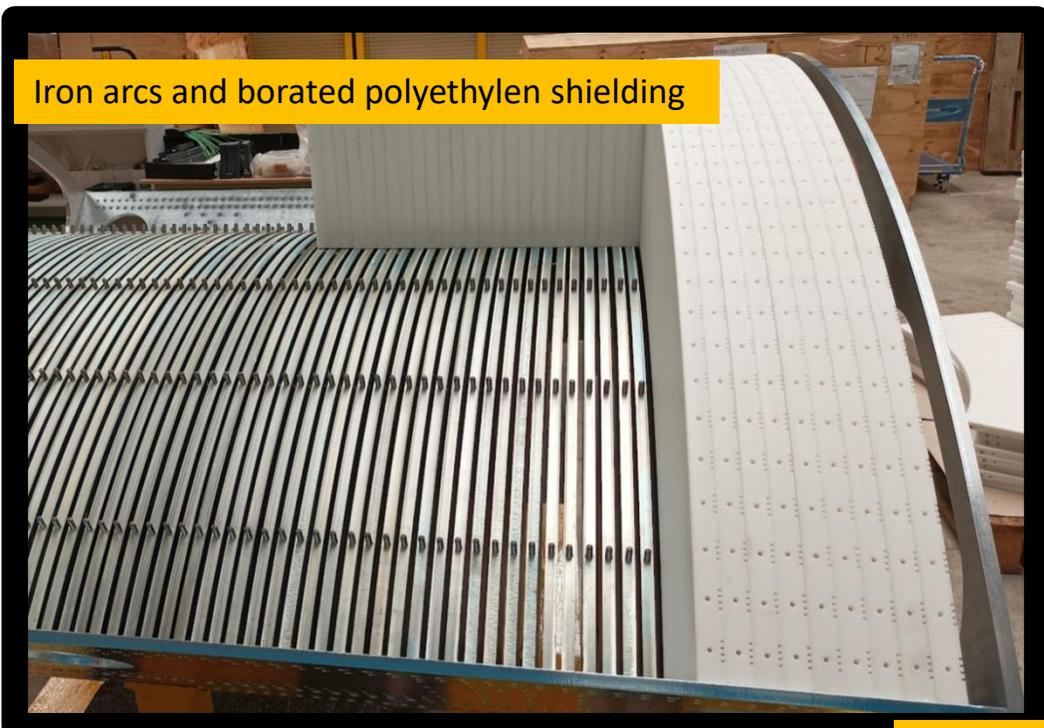
Iron arcs and borated polyethylene shielding
