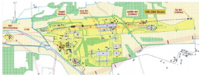
Figure 1. The new SPS North Area neutrino beam layout. Main parameters are: primary beam : 100 GeV; fast extracted from SPS; target station next to TCC2, ~11m underground; decay pipe: 100m, 3 m diameter; beam dump : 15m of Fe with graphite core, followed by muon stations; neutrino beam angle: pointing upwards; at -3m in the far detector ~5mrad slope. From I. Efthymiopoulos / CERN.
