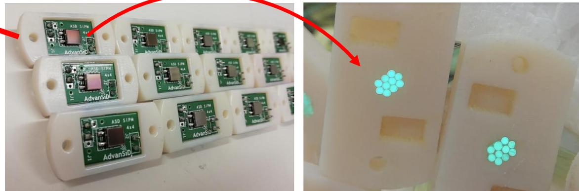
SiPMs installed outside of calorimeter, above shielding: avoid hadronic shower and reduce (factor 18) aging
