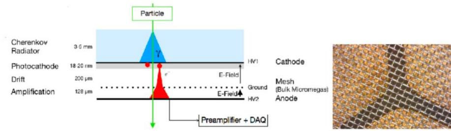
**Possible candidates:** fast Micromegas detectors with Cherenkov radiators (PIMENT)
